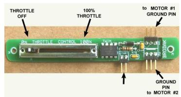
In a twin-motor installation, both motors receive the same throttle value but you can increase the line tension if you making the pitch of the inboard prop slightly greater, so it has more thrust.
